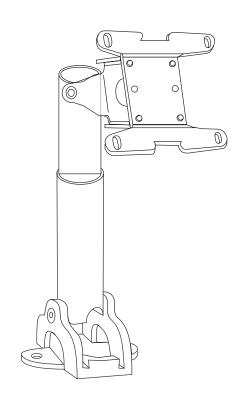
Typical Pedestal Type Mount with Swivel Bracket
